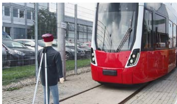
The system detects obstacles, assesses the risk of collision in real time and warns drivers of potential hazards.
