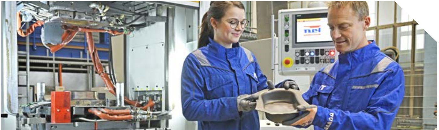
Experts at the LKR Leichtmetallkompetenzzentrum Ranshofen are implementing an innovative process for deep drawing titanium sheets.
